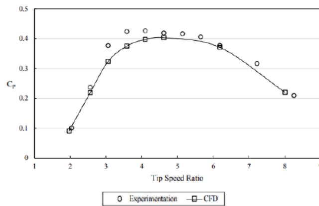
Figure 3 – Power Coefficient with TSR for Three-Bladed Turbine
